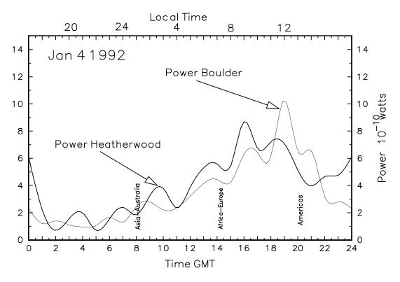
Fig. 55. Diurnal variations in specific power at two different locations on June 4 1992.
