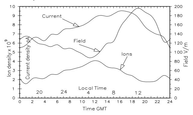
Fig. 49. Diurnal variations of electric field, ion current and ion density from 16 fairweather days in Dec. 1990.
