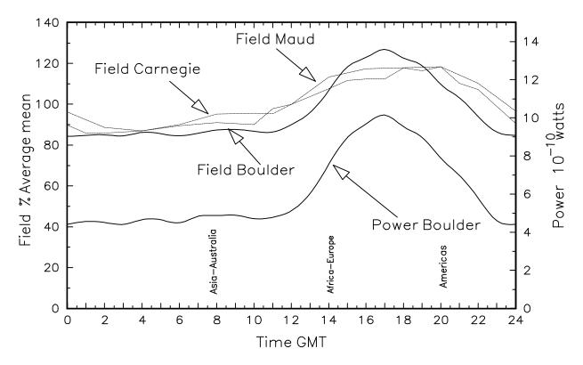
Fig. 54. Diurnal variations in electric field and power generated in Boulder compared to field variations from the Carnegie and Maud expeditions.
