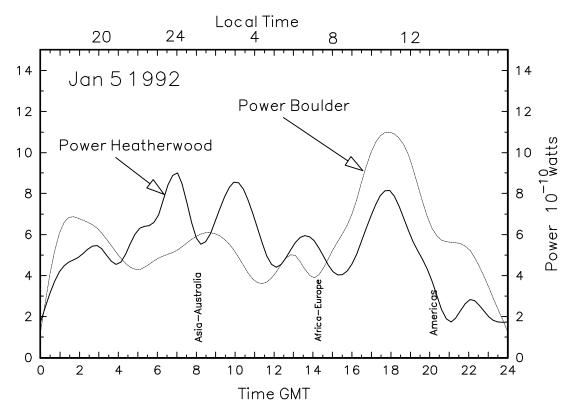
Fig. 56. Diurnal variations in specific power at two different locations on June 5, 1992.
