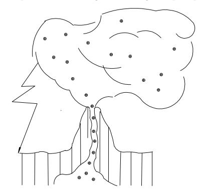
Fig. 37 Electrostatic charging of volcanic plume.
