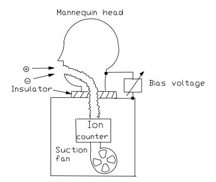
Fig. 39 Apparatus intake through the respiratory system.
