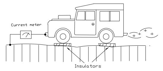
Fig. 36 Exhaust charging of a motor car.
