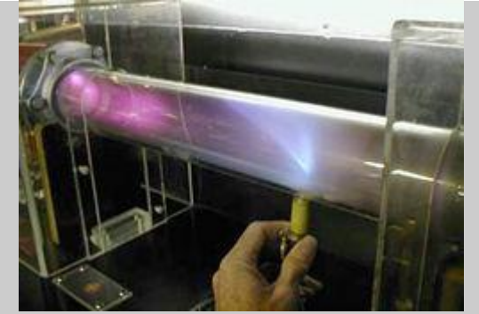
A glow discharge tube with a magnet showing the red anode column and blue filaments.
